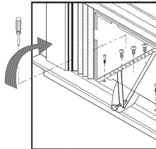
Use a wood block between the leveling bolts and the wall if the wall is weak or if the weight of the air conditioner falls between the studs in the wall.
