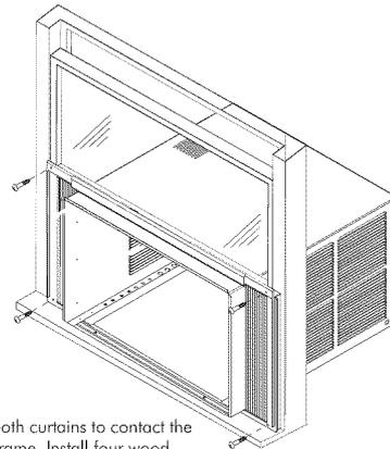
Expand both curtains to contact the window frame. Install four wood screws 31/32". Two in each upper right and left of the curtains. Use three wood screws 31/32" to fix the case to windows sash.
