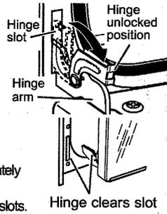
**NOTE:** The oven door is very heavy. Be sure you have a firm grip before lifting the oven door off the hinges. Use caution once the door is removed. Do not lay the door on its handle. This could cause dents or scratches.
