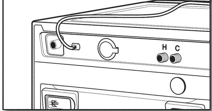
Remove the yellow shipping strap from the cord. Gently place power cord over top of washer to allow free access to back of washer.
