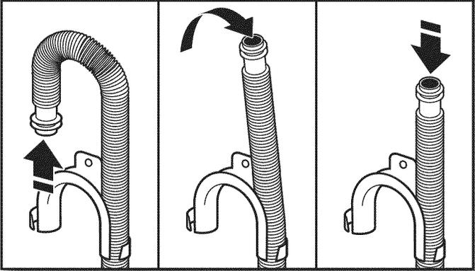
For floor drain installations, you will need to remove the drain hose form from the end of the drain hose. You may need additional parts with separate directions. See "Alternative Parts".
