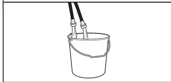
Run water for a few seconds through hoses into a laundry tub, drainpipe, or bucket to prevent clogs. Water should run until clear.
