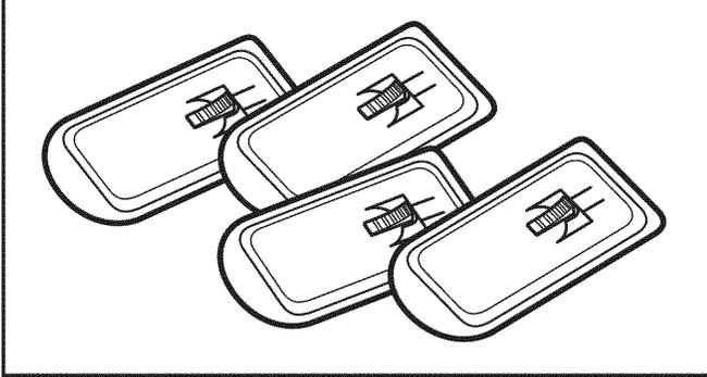
Close bolt holes on cabinet back with four transport bolt hole plugs included with washer parts.
