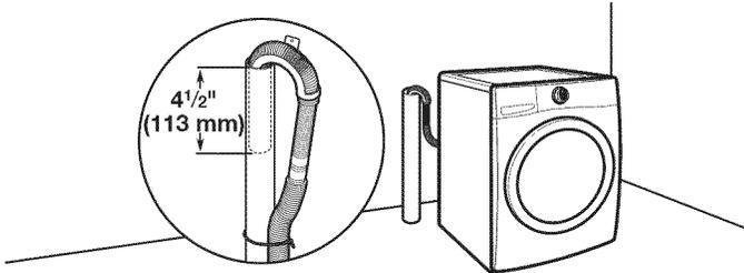
Minimum diameter for a standpipe drain: 2" (51 mm). Minimum carry-away capacity: 17 gal. (64 L) per minute. A 1/4" (6 mm) diameter to 1" (25 mm) diameter Standpipe Adapter Kit is available (Part Number 3363920). Top of standpipe must be at least 30" (762 mm) high; install no higher than 96" (2.44 m) from bottom of washer. If you have an overhead sewer and need to pump higher than 96 inches, a sump pump and associated hardware are needed. See "Alternative Parts".
