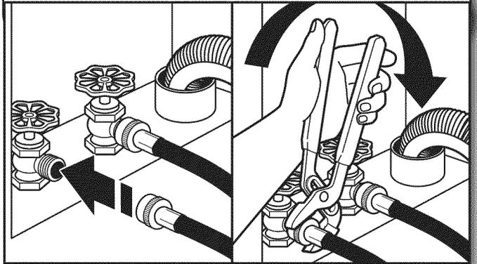
Attach hose to hot water faucet. Screw on coupling by hand until it is seated on washer. Use pliers to tighten couplings an additional two-thirds turn. Repeat this step with second hose for cold water faucet.
