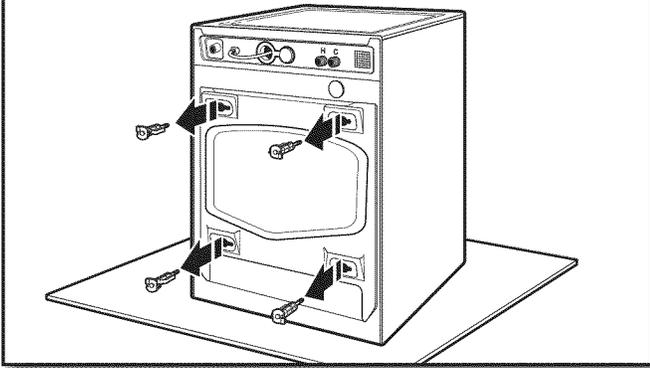
Loosen bolts with a 13 mm (1/2") wrench. Slide each bolt and spacer to center of hole. Pull bolts and plastic spacers from back of washer. Discard bolts and spacers.
