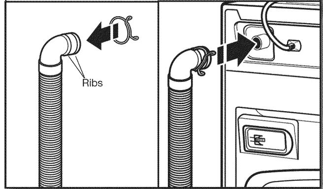
If clamp is not already in place on elbow end of drain hose, slide it over end of hose, centering it between the ribs, as shown. Squeeze clamp with pliers and slide elbow end of drain hose onto drain port and secure with clamp.
