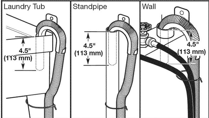
Secure drain hose to laundry tub leg, drain standpipe, or inlet hoses for wall standpipe with beaded tie strap.
