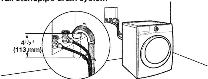
See requirements for floor standpipe drain system.
