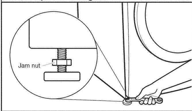
If washer is not level, use a 9/16" or 14 mm open-end or adjustable wrench to turn jam nuts clockwise on feet until they are about 1/2" (13 mm) from the washer cabinet. Then turn the leveling foot clockwise to lower the washer or counterclockwise to raise the washer. Recheck levelness of washer and that all four feet are firmly in contact with the floor. Repeat as needed.
