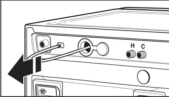
Pull power cord through opening in rear panel and close hole with attached cap.
