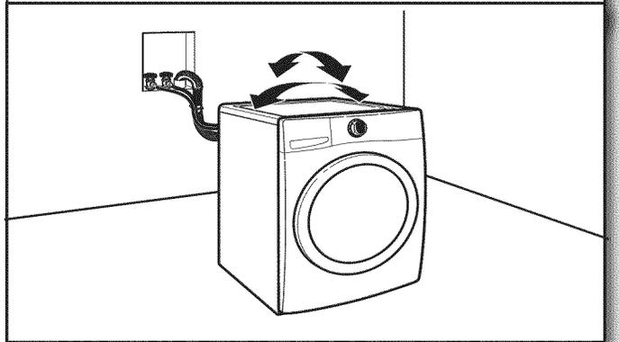
Grip washer from top and rock back and forth, making sure all four feet are firmly on floor. Repeat, rocking washer from side to side. If washer rocks, go to step 17 and adjust leveling feet. If all four feet are in firm contact with floor, go to Step 18.
