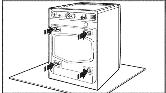
Locate four transport bolts on rear of washer.
