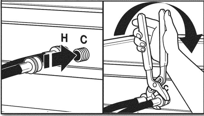
Attach hot water hose to hot water inlet valve marked with a red ring. Screw coupling by hand until it is snug. Use pliers to tighten couplings an additional two-thirds turn. Repeat with cold water inlet valve.
