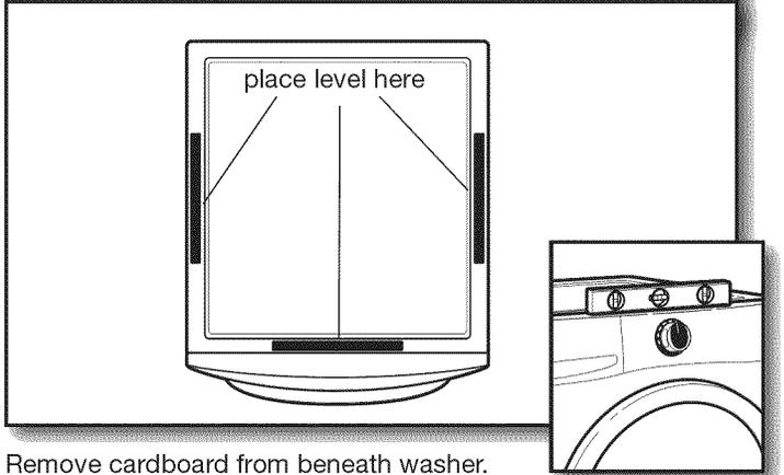
Remove cardboard from beneath washer. Place a level on top edges of washer, checking each side and front. If not level, tip washer and adjust feet up or down as shown in steps 17 and 18, repeating as necessary.
