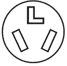
3-wire receptacle (10-30R)
