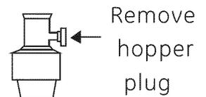
**TIP:** Avoid unnecessary service call charges. Always be sure disposer drain plug has been removed before attaching dishwasher drain hose to the disposer.
