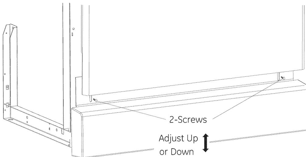
Install 2 toekick screws to fasten toekick. Allow the toe kick to tuch the floor.
