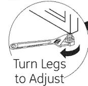
**TIP:** Pull lower rack out, about halfway. Check to be sure the rack does not roll forward or back into dishwasher. If the rack rolls in either direction, the dishwasher must be leveled again.
