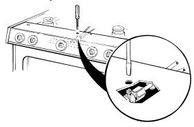
**ACAUTION** — Make sure the surface burner control knobs are in the **OFF** position before attempting to adjust the pilots.
