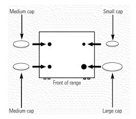
Make sure that the heads and caps are replaced in the correct locations.
