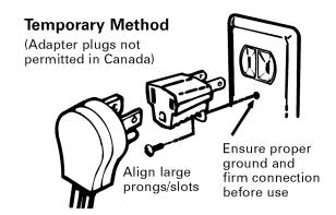
**ACAUTION** — Attaching the adapter ground terminal to the wall receptacle cover screw does not ground the appliance unless the cover screw is metal, and not insulated, and the wall receptacle is grounded through the house wiring. The customer should have the circuit checked by a qualified electrician to make sure the receptacle is properly grounded.
