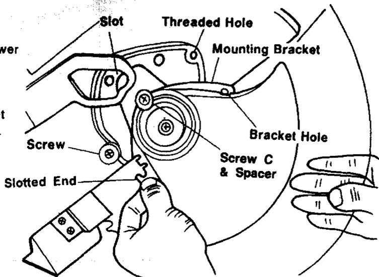
6. Replace screw B, that was removed in step 3. Tighten screw A and screw B.
