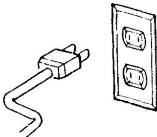
This power tool is equipped with a 2-conductor cord listed by Underwriters Laboratories (UL). The plug permits you to use any conventional 120-volt electrical outlet without necessity for maintaining a ground connection.
