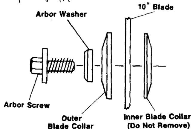
**WARNING:** After installing a new blade, make sure the blade clears the table slot at the 0° and 45° bevel positions. Lower the blade into the lower table and check for any contact with the base or turn table structure.
