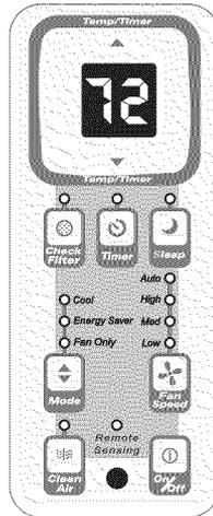
Note: Tap or hold either up (▲) or down (▼) button until the desired temperature is seen on the display. This temperature will be automatically maintained anywhere between 60 °F (16 °C) and 90 °F (32 °C). If you want the display to read the actual room temperature. See "To Operate on Fan Only" section on Page 6.
