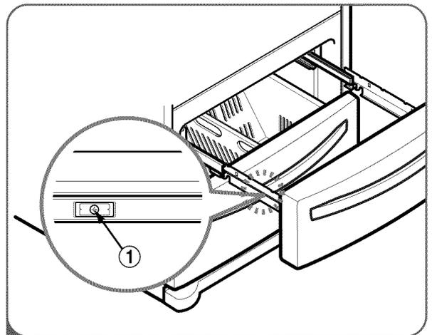
2 Remove one white screw ① on each side of the rails.
