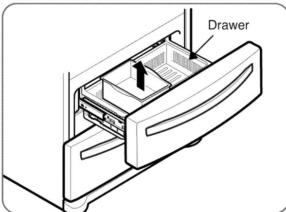
To separate the ice bin, pull out the drawer to full extension. Gently lift and pull out the ice bin. To reinstall, simply set the ice bin in its correct position.
