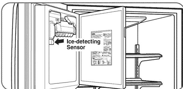
**NOTE:** Avoid touching the Ice-detecting sensor when replacing the ice bin. See the label on the ice compartment door for details.
