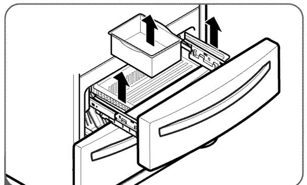
4 With both hands, bend the center bar just enough to allow the gears on both ends to release from their tracks.
