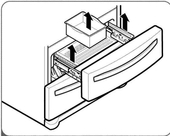
1 Fully extend the freezer drawer. Lifting up and out to remove the drawer and ice bin making sure to clear the rail system.
