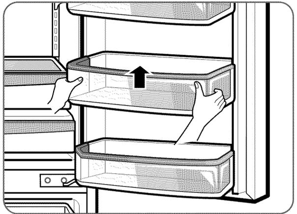
The door bins are removable for easy cleaning and adjusting. Simply lift the bin and pull it straight out to remove it. To replace the bin, slide it in above the desired support button and push down until it stops.
