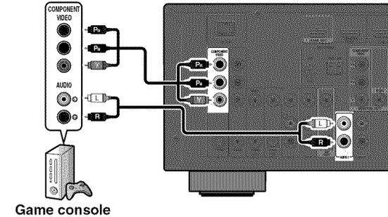
You can use the video input from the AV1-2 jacks in combination with the audio input from other AV inputs or AUDIO1-2.
