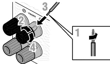
**1** Remove approximately 10 mm of insulation from the ends of the speaker cables, and twist the bare wires of the cables together firmly so that they will not cause short circuits.
