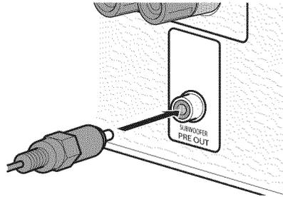
**1** Connect the subwoofer input jack to the SUBWOOFER jack on this unit with an audio pin cable.
