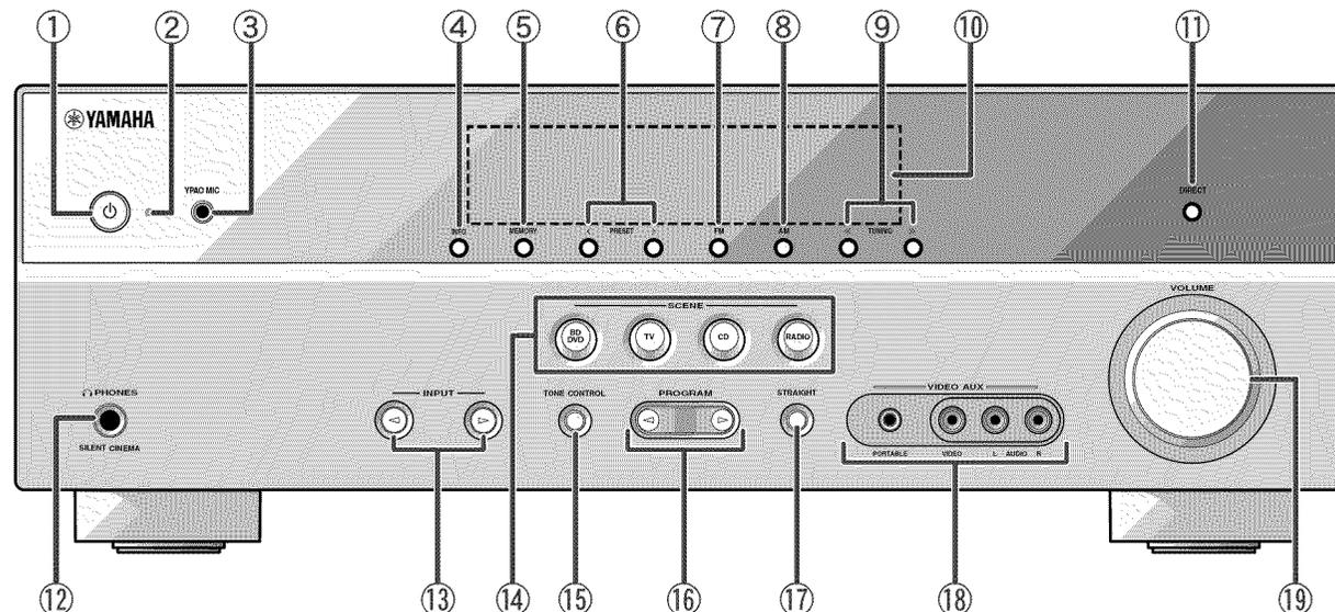
1 : During the standby mode, you can select the HDMI input (HDMI1-4) to output to a TV. When the input is changed correctly, HDMI Through/iPod Charge indicator blinks twice.
