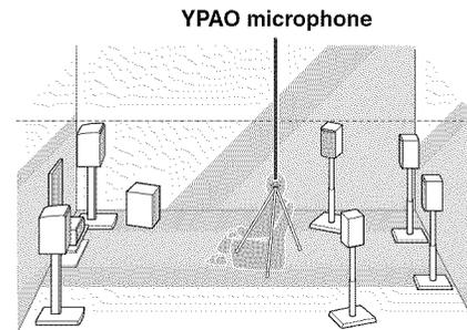
When positioning the microphone, we recommend that you use equipment that allows you to adjust the height (such as a tripod) as a microphone stand. When using a tripod, use the tripod screws to fix the microphone in place.
