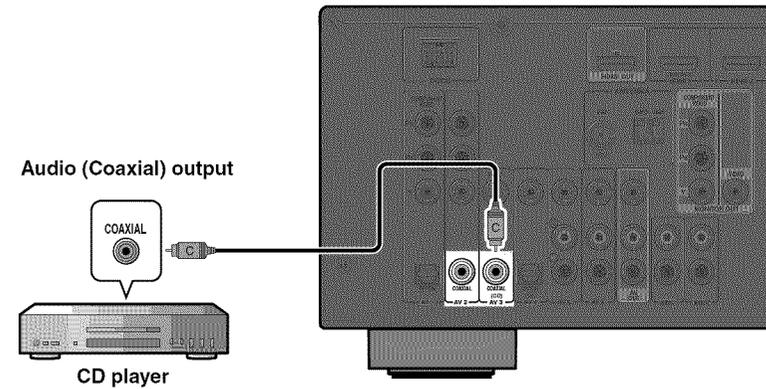
We recommend connecting audio devices with an coaxial digital output to the AV3 coaxial digital jack on this unit. This connection allows you to switch to the AV input 3 just by pressing the “CD” SCENE key (see p. 30).
