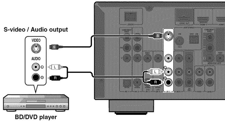
Select the AV5 input source for connected video output that the playback device is connected to for playback. Video from the S VIDEO jack is output through the HDMI OUT jack only.
