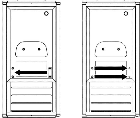
3. Push the hole plugs into place on the opposite side of the door.
