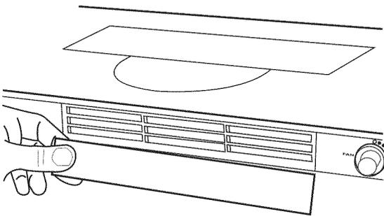
4. Lift the range hood up under cabinet and determine final location by centering beneath cabinet. Mark on the underside of cabinet the location of the 4 keyhole mounting slots on the range hood. Set range hood aside on a covered surface.
