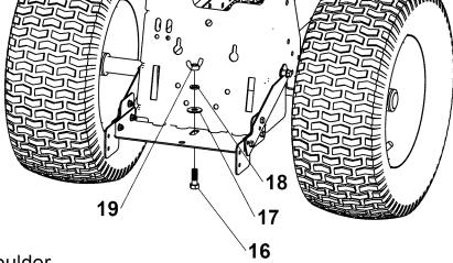
Hook Tractor Brackets onto shoulder bolts and secure Center Plate to tractor with hardware as shown. **Assembly Instructions**
