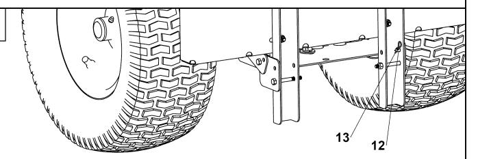
Secure in upright position using Clevis Pin and Hairpin as shown.
