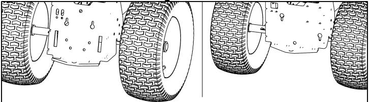
Identify your tractor model before assembling this product. Garden Tractors have sloped backs as shown on the left. Lawn Tractors have vertical backs as shown on the right.
