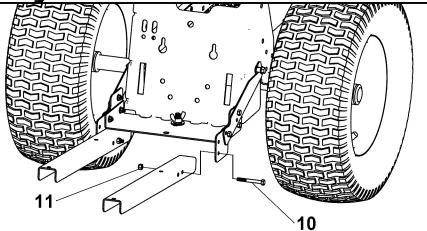
Attach Support Arms to Side Plates as shown. Do not tighten nut completely, arms must freely rotate.
