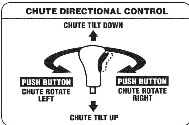
The chute directional control is located on the left side of the dash panel.
