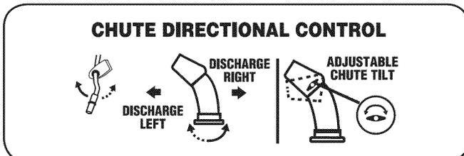
The chute directional control is located on left side of the snow thrower. To change the direction in which snow is thrown, rotate the chute directional control.
