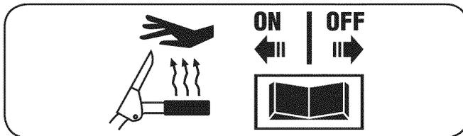
To activate the heated grips, move the switch found on the rear of the dash panel into the ON position.
