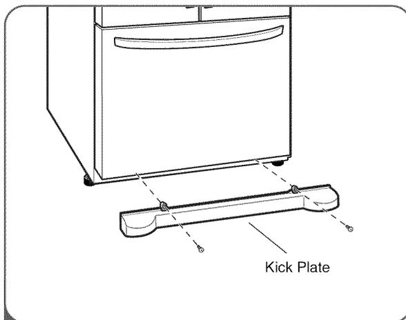
1 Plug the power cord into a 3-prong grounded outlet, and move the refrigerator into its final position. Remove the kick plate screws and then the kick plate.
