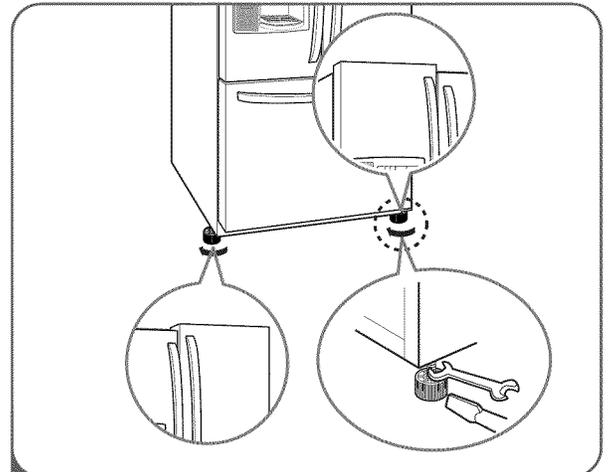
2 Level the refrigerator by using an 11/16 inch (18mm) wrench or a flat blade screw driver. Turn the leveling legs (CCW) to raise or (CW) to lower the height of the front of the refrigerator.
