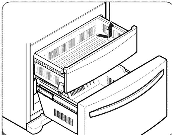
1 To remove the drawer, push the tabs located on the front inside surface of each rail. Next, gently lift the rear left and right sides of the drawer and pull it out.
