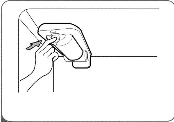
1 Press the push button to open the filter cover.
