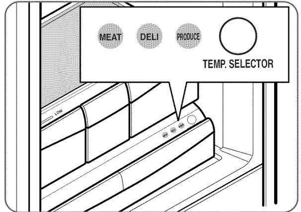
The Glide'N'Serve provides storage space with a variable temperature control that keeps the compartment colder than refrigerator.
