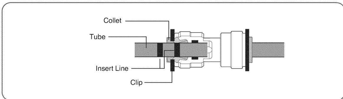
1. Insert the tube until you can see only one of the lines printed on the tube.
