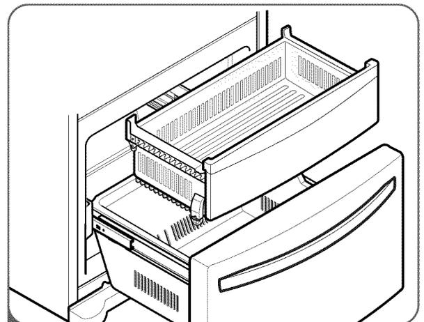
2 To reinstall, pull out and fully extend both rails. Insert the end of rib in the bracket at left and right. Making sure that the guides at the front are lined up properly, gently push down on both sides.
