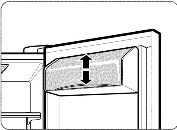
To remove the dairy bin, simply lift it and pull straight out. To replace the dairy bin, slide it into place and push down until it stops.
