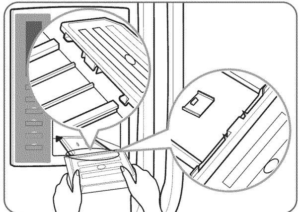
The dispenser drip tray has no self-draining function. It should be cleaned regularly. Remove the cover by pressing and pulling the tray. Dry it with a cloth. To reinstall the tray, slightly tilt the front of the tray and snap the ribs into the holes.
