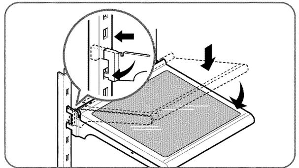
Tilt up the front of the shelf and guide the shelf hooks into the slots at a desired height. Then lower the front of the shelf so that the hooks drop into the slots.
