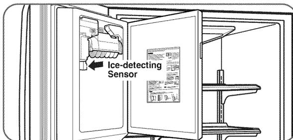
**NOTE:** Avoid touching the Ice-detecting sensor when replacing the ice bin. See the label on the ice compartment door for details.
