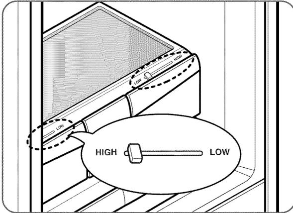
You can control the amount of humidity in the moisture-sealed crispers. Store vegetables or fruits requiring more or less humidity in separate crispers. Adjust the control to any setting between HIGH and LOW.
