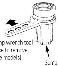
Turn sump wrench tool clockwise to remove (on some models)
