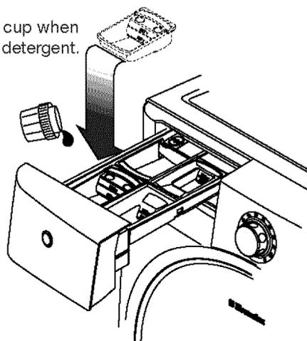
Remove liquid cup when using powder detergent! DO NOT pour powder detergent into liquid cup. It will not dispense correctly!
