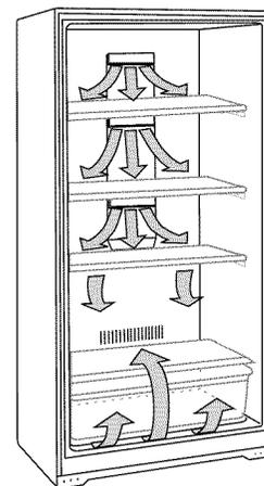
Do not block any of these vents with food packages. If the vents are blocked, airflow will not occur, and temperature and moisture problems may occur.
