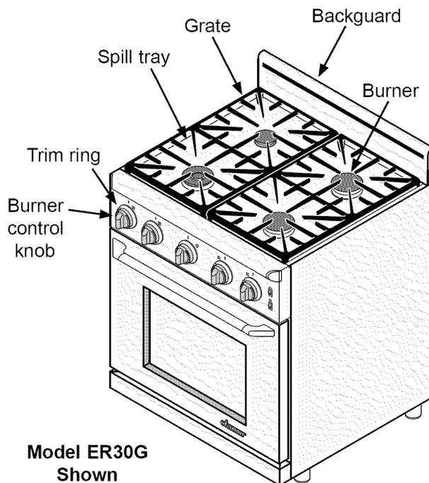
Model ER30G (freestanding model) is equipped with full size stainless steel side panels. Model ER30GI is equipped with three inch deep side panels. It is designed for installation in a recessed cabinet or island.
