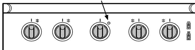
2. For best results, do not place food inside the oven until the oven has preheated to the set temperature. When pre-heated to the set temperature, the oven ON indicator light will begin to turn on and off every few seconds, because the set temperature has been reached and the oven is maintaining it.
