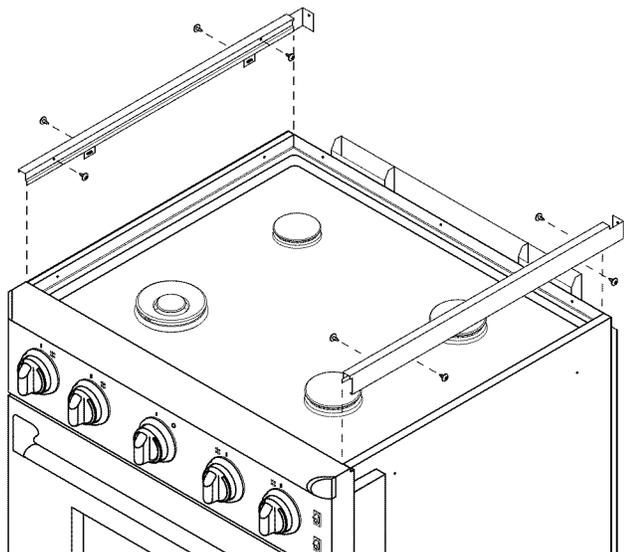
5. Slide the provided left and right trim pieces onto the range. The overhang on each piece goes toward the back.
