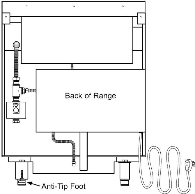
2. Locate the anti-tip bracket included in the parts box.
