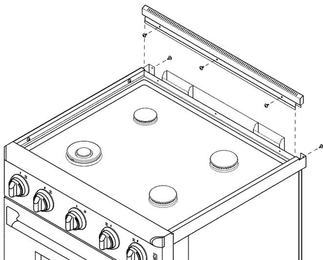
3. Remove and discard the screws (4 each) that hold the existing left and right trim pieces in place.
