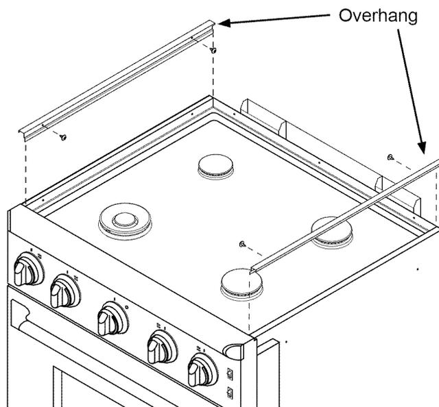
7. Reattach the backguard using three (3) of the #8 x 1/4" Torx screws.
