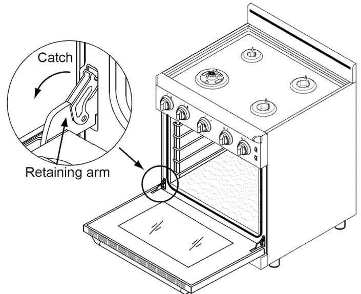
3. Lift the oven door to about a 15° angle from the vertical position.
