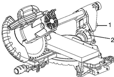
**NOTE:** The saw comes with a 33.9° crown molding stop.
