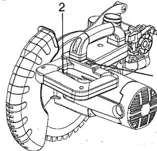
Your tool is equipped with the Laser Trac® cutting guide using a Class IIIa laser beam. The laser beam allows you to preview the saw blade path on the stock to be cut before starting the miter saw. This laser guide is powered by the transformed alternating current supply directly through the power lead. **The saw must be connected to the power source and the laser on/off switch must be turned on for the laser line to show.**
