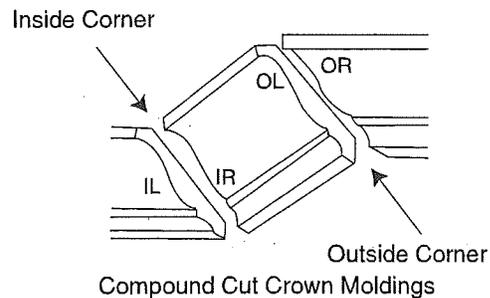
**NOTE:** The chart on next page references a compound cut for crown molding **ONLY WHEN THE ANGLE BETWEEN THE WALLS EQUALS 90°.**
