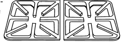
**Do not operate the burners without a pan on the grate. The grate's porcelain finish may chip without a pan to absorb the heat from the burner flame.**
