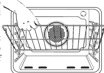
**To replace:** Place rack on the rack support in the oven; tilt the front end up slightly; slide rack back until it clears the lock-stop position; lower front and slide back into the oven.
