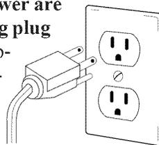
The three-prong grounding plug offers protection against shock hazards. **DO NOT CUT OR REMOVE THE THIRD GROUNDING PRONG FROM THE POWER CORD PLUG.**
