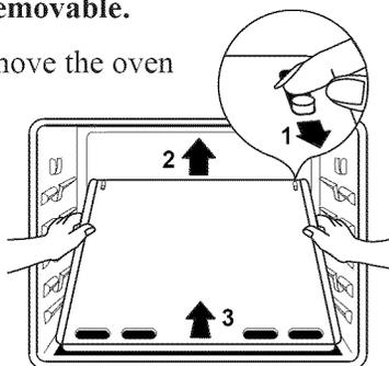
edge of the oven bottom clears the oven front frame. Remove oven bottom from oven.
