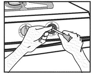
**To adjust:** Operate burner on HIGH for about five minutes to preheat burner cap. Turn knob back to LOW; remove knob, and insert a small screwdriver into the center of the valve stem. Adjust the flame size by turning adjustment screw in either direction, while holding the stem.
