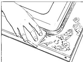
**To prevent damage, do not clean or rub the gasket around the oven door.** The gasket is designed to seal in heat during the clean cycle.
