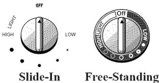
Use to turn on the surface burners. An infinite choice of heat settings is available from LOW to HIGH. At the HIGH setting a detent or notch may be felt. The
