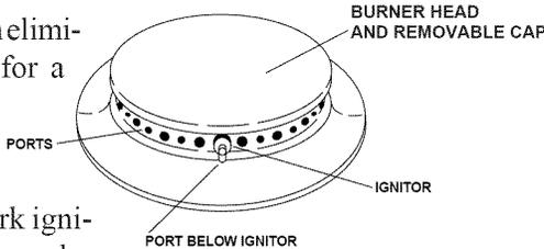
If the surface burner does not light, check if ignitor is broken, soiled or wet. If clogged, clean the small port beneath the ignitor using straight pin.
