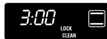
5. When the cleaning time has been completed, the indicator word CLEAN will turn off. The indicator word LOCK will remain on until the oven has cooled (approx. 1 hour). When the oven has cooled, the indicator word LOCK will turn off and the door will automatically unlock.
