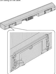
Loop the safety wires (not supplied) into each hole as shown and tie the safety wires to the LCD TV stand.
