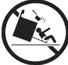
To reduce the risk of tipping of the range, the range must be secured by properly installed anti-tip bracket(s) provided with the range. To check if the bracket (s) is installed properly, remove the lower panel or storage drawer and verify that the anti-tip bracket (s) is engaged. Refer to the installation instructions for proper anti-tip bracket(s).
