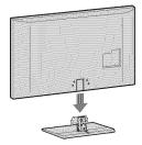
**2** Use the supplied screws to attach the TV unit to the Table-Top Stand.
