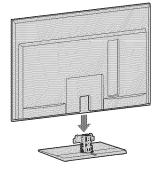
**2** Use the supplied screws to attach the TV unit to the Table-Top Stand.
