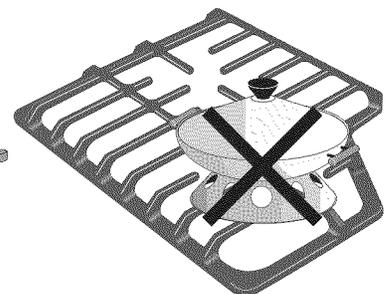
Improper use of round-bottom wok on Surface Burner Grate
