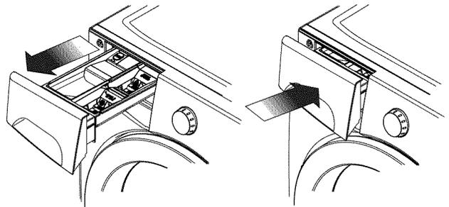
Insert liquid cup when using liquid detergent.
