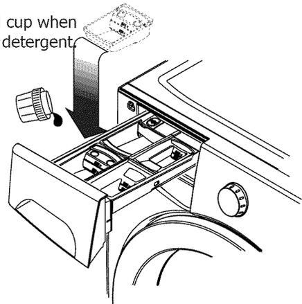
Remove liquid cup when using powder detergent! **DO NOT** pour powder detergent into liquid cup. It will not dispense correctly!
