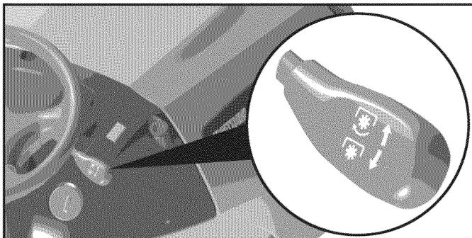
(☒) ATTACHMENT CLUTCH LEVER "DISENGAGED"
