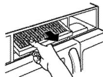
5. **Slide** a new charcoal filter into place. The filter should rest at the angle shown.
