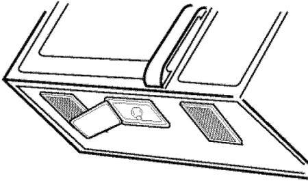
2. Remove the bulb cover mounting screws.
