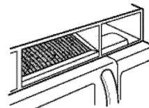
6. **Slide** the bottom of the vent grille into place. **Push** the top until it snaps into place. **Replace** the mounting screws.
