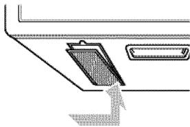
4. To replace grease filters, slide filter in the frame slot on one side of the opening. Push filter upward and push to the other side to lock into place.
