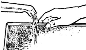
3. Soak grease filters in hot water and a mild detergent. Scrub and swish to remove embedded dirt and grease. Rinse well and shake to dry. Do not clean filters with ammonia, corrosive cleaning agents such as lye-based oven cleaners, or place them in a dishwasher. The filters will turn black or could be damaged.
