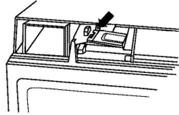
6. Lift up the bulb holder and slide out of compartment.
