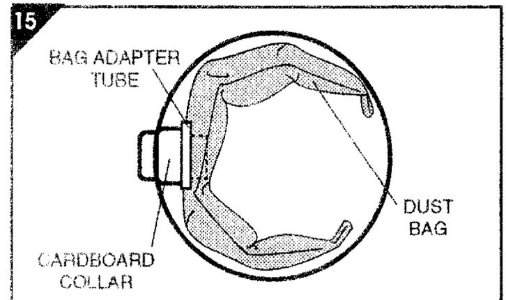
**CAUTION: PAPER DUST BAG IS FOR DRY PICK UP ONLY. DO NOT USE WHEN VACUUMING LIQUIDS!**
