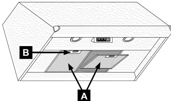
2. While pushing back on the release lever, lower the filter out of the hood. On hoods with more than one filter, remove and clean all of the filters.
