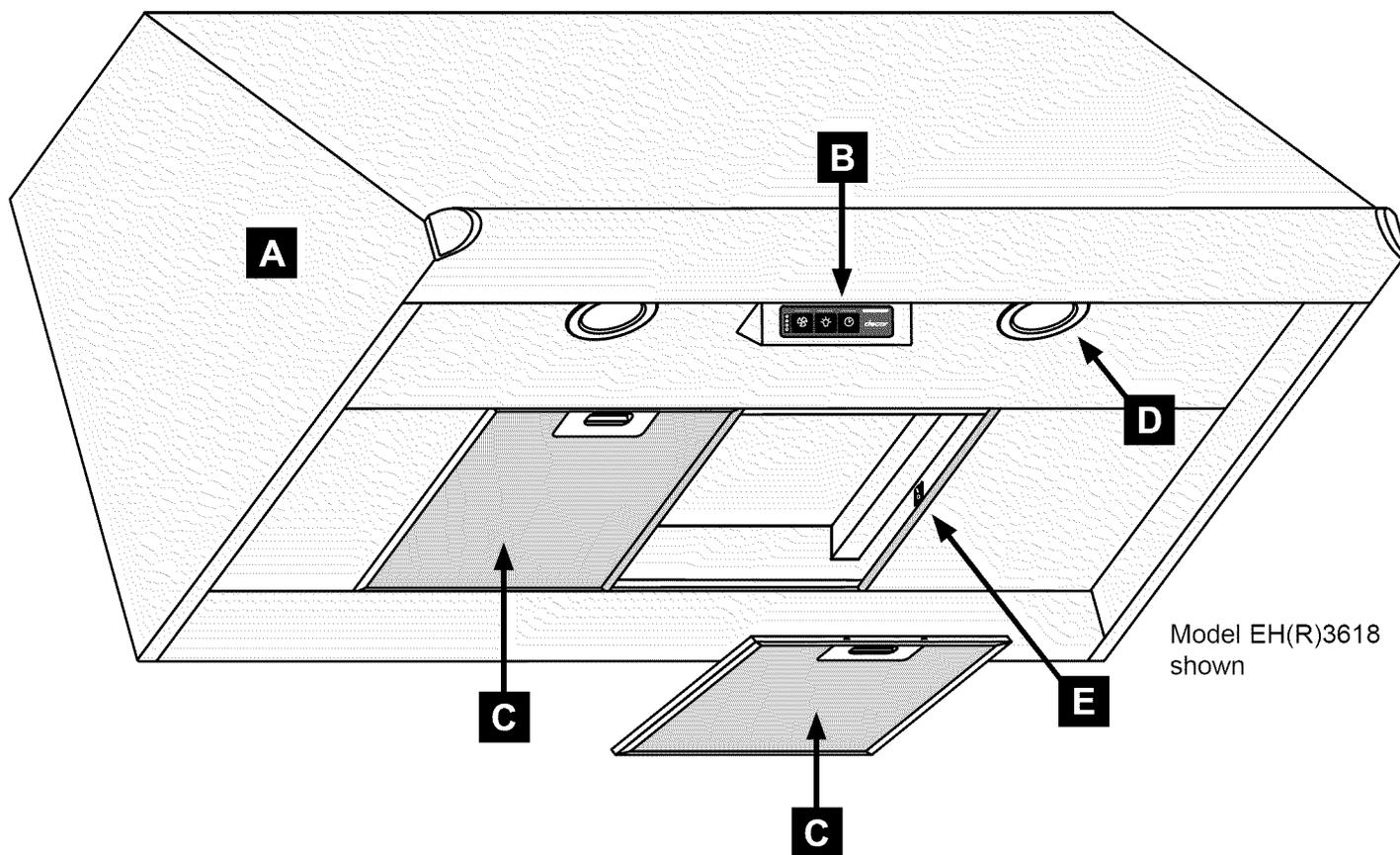
**A HOOD** - The hood directs heat and smoke into the fan located inside the unit. The fan forces heat and smoke into the duct system which vents to the outside. The filter and the lights are located on the bottom of the hood.
