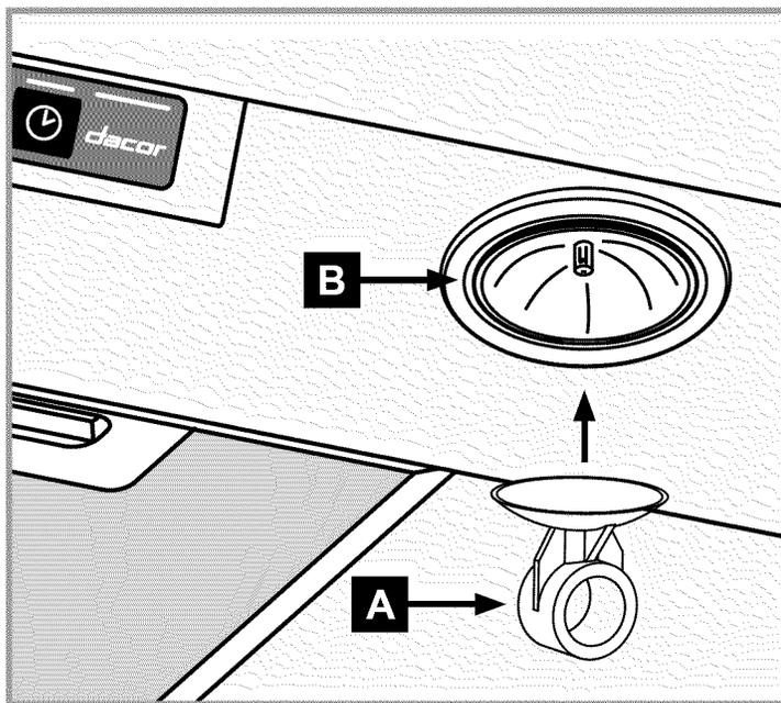
3. Turn the tool counter-clockwise until the bulb comes loose.
