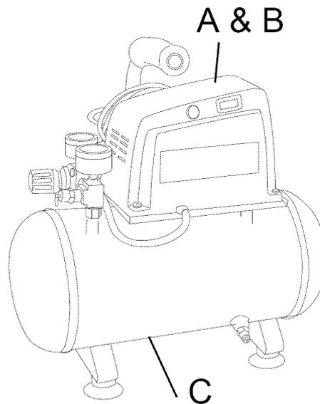
The pump (see B) compresses the air and discharges it into the tank.
