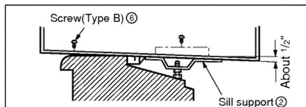
7. Attach the cabinet to the window stool by driving the screws ⑥(Type B: Length sixteen millimeters and below.) through the front angle into window stool.
