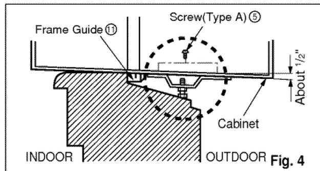
5. Attach the sill support to the cabinet track hole in relation to the selected position using 2 Type A screws in each support(See Fig. 4).
