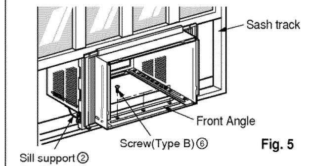
8. Pull each Frame curtain fully to each window sash track, and repeat step 2.
