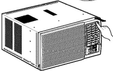
The direction of air can be controlled wherever you want to cool by adjusting the horizontal louver and the vertical louver.
