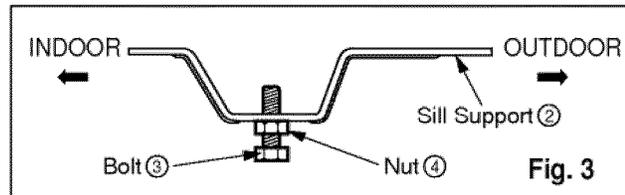
4. Select the position that will place the sill support near the outer most point on sill (See Fig. 4)
