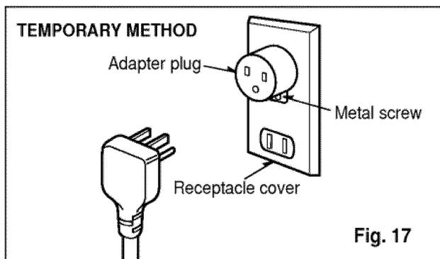
Because of potential safety hazards, we strongly discourage the use of an adapter plug. However, if you wish to use an adapter, a TEMPORARY CONNECTION may be made. Use UL-listed adapter, available from most local hardware store(Fig. 17). The large slot in the adapter must be aligned with the large slot in the receptacle to assure a proper polarity connection.
