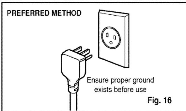
**DO NOT CUT OR REMOVE THE THIRD(GROUND) PRONG FROM THE POWER PLUG.**
