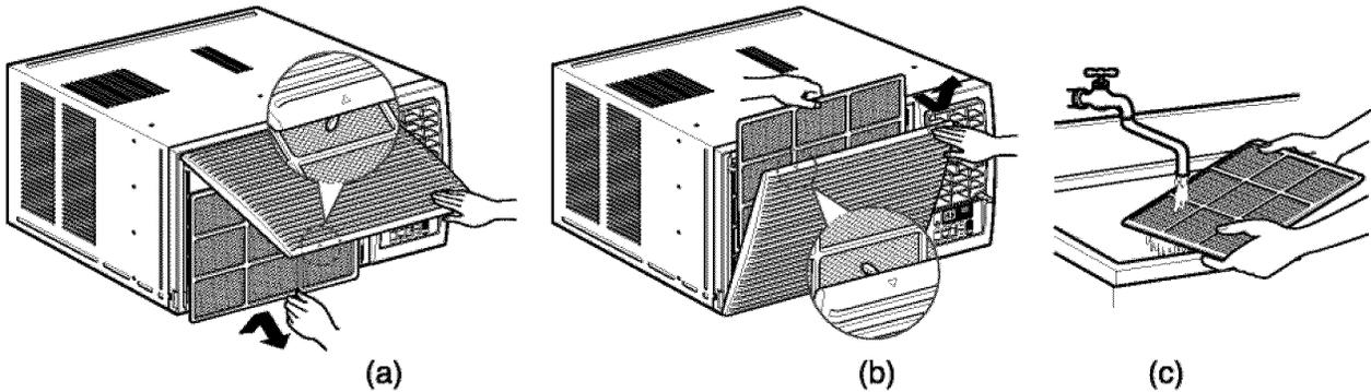
**CAUTION:** DO NOT operate the air conditioner without a filter because dirt and lint will clog it and reduce performance.
