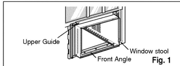
2. Pull the bottom window sash down behind the upper guide until it meets.
