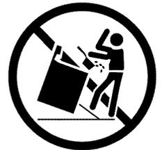
For models equipped with a warmer drawer or lower oven, grasp the top rear edge of the range and carefully attempt to tilt it forward. Refer to the installation instructions for proper anti-tip bracket installation.
