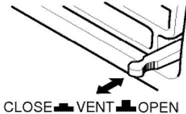
**NOTE :** Before using the ventilation feature, position the vent lever straight by pulling Part A out and snapping it into place.
