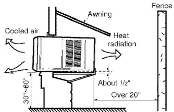
**CAUTION:** All side louvers of the cabinet must remain exposed to the outside of the structure.
