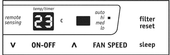
Note: Tap or hold either up ( **A** ) or down ( **V** ) button until the desired temperature is seen on the display. This temperature will be automatically maintained anywhere between 16 °C (60 °F) and 32 °C (90 °F) . If you want the display to read the actual room temperature. See "To Operate on Fan Only" section on Page 6.
