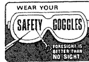
Any power saw can throw foreign objects into the eyes. This can cause permanent eye damage. Wear safety goggles (not glasses) that comply with ANSI Z87.1 (shown on package). Everyday eyeglasses have only impact resistant lenses. They are not safety glasses. Safety goggles are available at Sears Retail or Catalog Stores. Glasses or goggles not in compliance with ANSI Z87.1 could seriously hurt you when they break.
