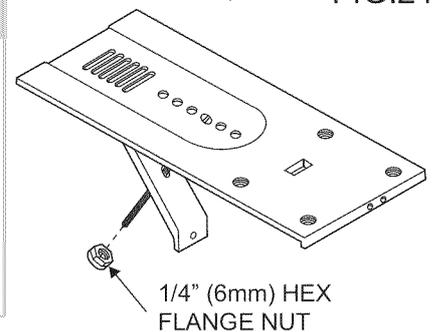
**24** Attach support brace to platform as shown (FIG.21). Use the adjustment bolt and hex flange nut to complete the assembly. Choose the slot and adjustment bolt hole location that will create a 45 degree angle between the platform and support brace. Try the assembly in the window to determine if the platform will rest properly, and allow the proper slope (3/16" lower on outside).
