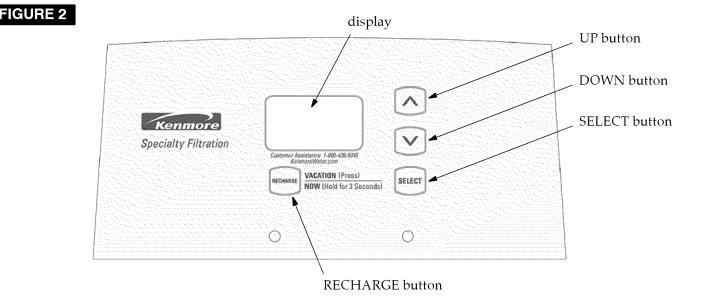
When the transformer is plugged into the electrical outlet a model code is displayed for a few seconds followed by a test number (example: J1.1). Then, 12:00 PM and the words PRESENT TIME will begin to flash in the time display.
