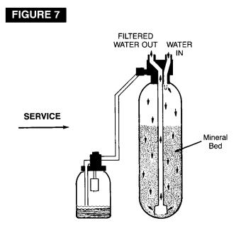
**IMPORTANT:** Avoid using water in the house while the filter is regenerating. Bypass iron water will go to house pipes and the water heater during the solution draw and backwash cycles if a faucet is opened.
