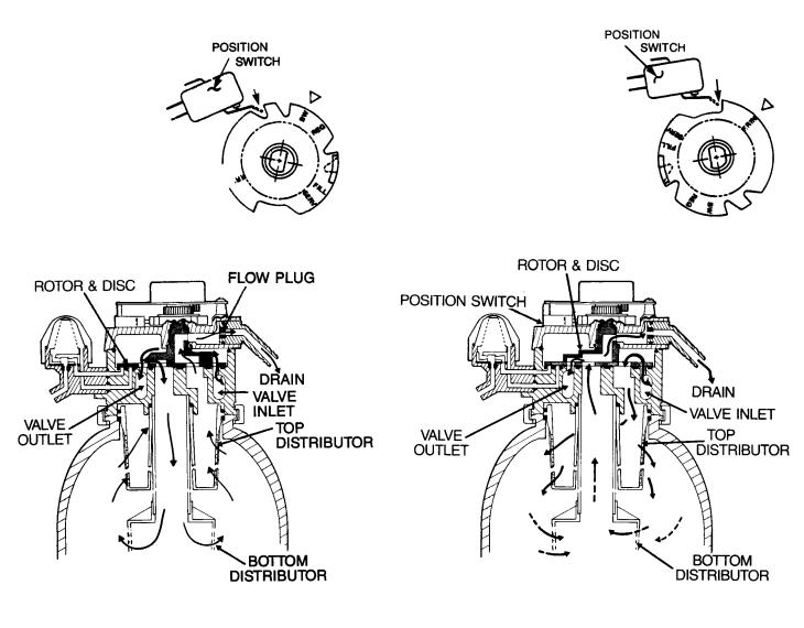
Switching action again allows the motor to turn the rotor & disc to place the valve in BACKWASH, stopping water flow to the nozzle. Water is routed down and out the bottom distributor, up through the bed, and out the top distributor to the drain. The fast flow (controlled by a flow plug in the drain fitting) flushes dirt, sediments, iron deposits, and remaining solution to the drain.
