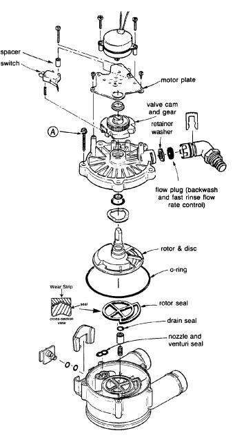
Tighten the screws using a criss-cross pattern. If a torque wrench is available, torque to 30-40 inch pounds.
