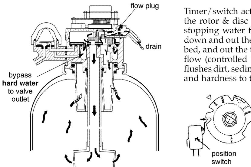
Timer/switch action again allows the motor to turn the rotor & disc to place the valve in BACKWASH, stopping water flow to the nozzle. Water is routed down and out the bottom distributor, up through the bed, and out the top distributor to the drain. The fast flow (controlled by a flow plug in the drain fitting) flushes dirt, sediments, iron deposits, remaining brine and hardness to the drain.
