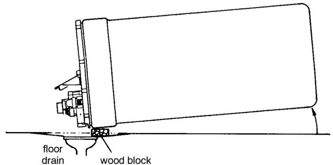
7. Looking at FIG. 11, lay a piece of 2 inch thick board near the floor drain. Move the softener close to the drain. SLOWLY and CAREFULLY, tip it over until the rim rests on the wood block with the inlet and outlet over the drain. **Do not allow the softener's weight to rest on the inlet and outlet fittings or they will break.**
