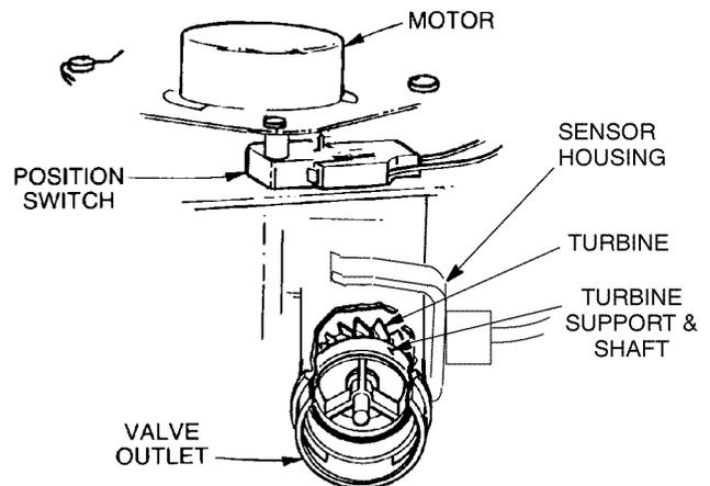
**POSITION SWITCH STATUS:** With the valve in service, or any of the recharge cycles, the switch indicator will show open  $\curvearrowright$ . While the valve is rotating from 1 position to another, the indicator will show the switch closed  $\curvearrowleft$ . A defect is probable if indications vary from this pattern.
