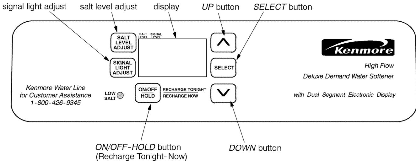
When the transformer is plugged in, the model code HF31, and a test number (example: k11) show in the face plate display for 4 seconds. Then, 12:00 AM and *PRESENT TIME* begin to flash.
