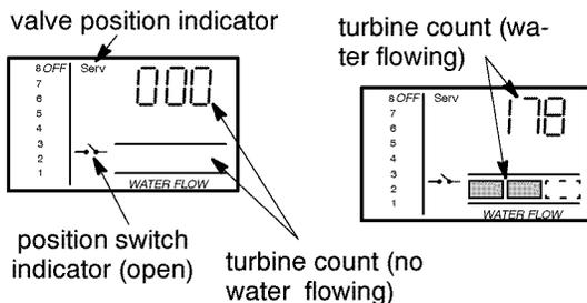
**TURBINE OPERATION:** If no water is flowing through the softener, the turbine indicator displays 3 zeros. When water is flowing, the flow bar scrolls across the display, and a 000 to 140 count repeats for each gallon of water passing through the turbine. To check for positive operation of the turbine if zeros are shown, open a nearby soft water faucet and observe the turbine count and flow bar.
