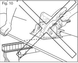
**Never** place the saw on the part of the workpiece that will fall off when the cut is made.
