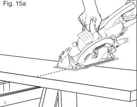
**A WARNING:** If the blade comes in contact with the workpiece before it reaches full speed, it could cause the saw to kickback towards you, possibly resulting in serious injury.
