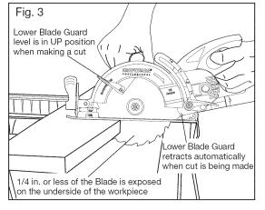
lower blade guard does not cover the blade on the underside of the workpiece. Keep hands and fingers away from the cutting area. If any part of your body comes in contact with the moving blade, serious injury will result.
