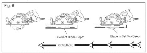
9. **Use extra caution** when making a "Pocket Cut" into existing walls or other blind areas. The protruding blade may cut objects that can cause Kickback.
