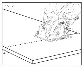
until the blade comes to a complete stop. **Never** attempt to remove the saw from the workpiece or pull the saw backward while the blade is in motion, or kickback may occur. Check and take corrective action to eliminate the cause of blade binding.
