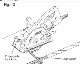
When using the edge guide, position the face of the edge guide firmly against the edge of the workpiece. This will help to make a true cut without binding the blade. The edge of the workpiece must be straight for the cut to be straight. Use caution to prevent the blade from binding in the cut.
