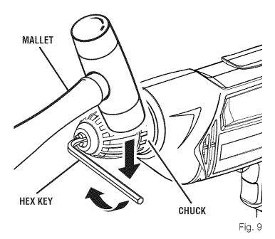
Open the chuck jaws and remove the hex key. Using a screwdriver, remove the chuck screw by turning it in a clockwise direction.
