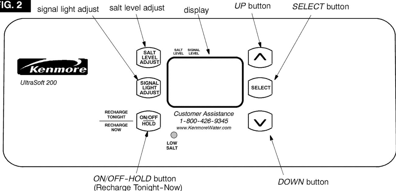
When the transformer is plugged in, the model code SR27, and a test number (example: k20) show in the face plate display for 4 seconds. Then, 12:00 AM and PRESENT TIME begin to flash.
