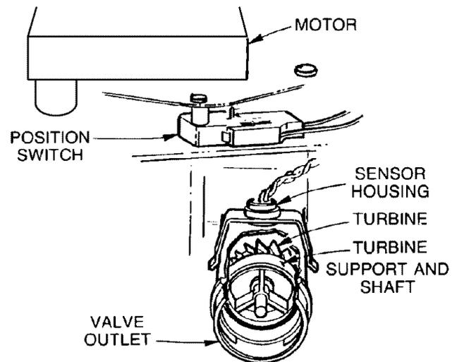
**POSITION SWITCH STATUS:** With the valve in service, or any of the recharge cycles, the switch indicator will show open  $\rightarrow$ . While the valve is rotating from 1 position to another, the indicator will show the switch closed  $\leftarrow$ . A defect is probable if indications vary from this pattern.
