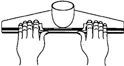
2. Using both hands, position each thumb on the removable insert, (below the latches) and two fingers of each hand on each latch, lift and disengage the two latches from the tabs on the nozzle body.
